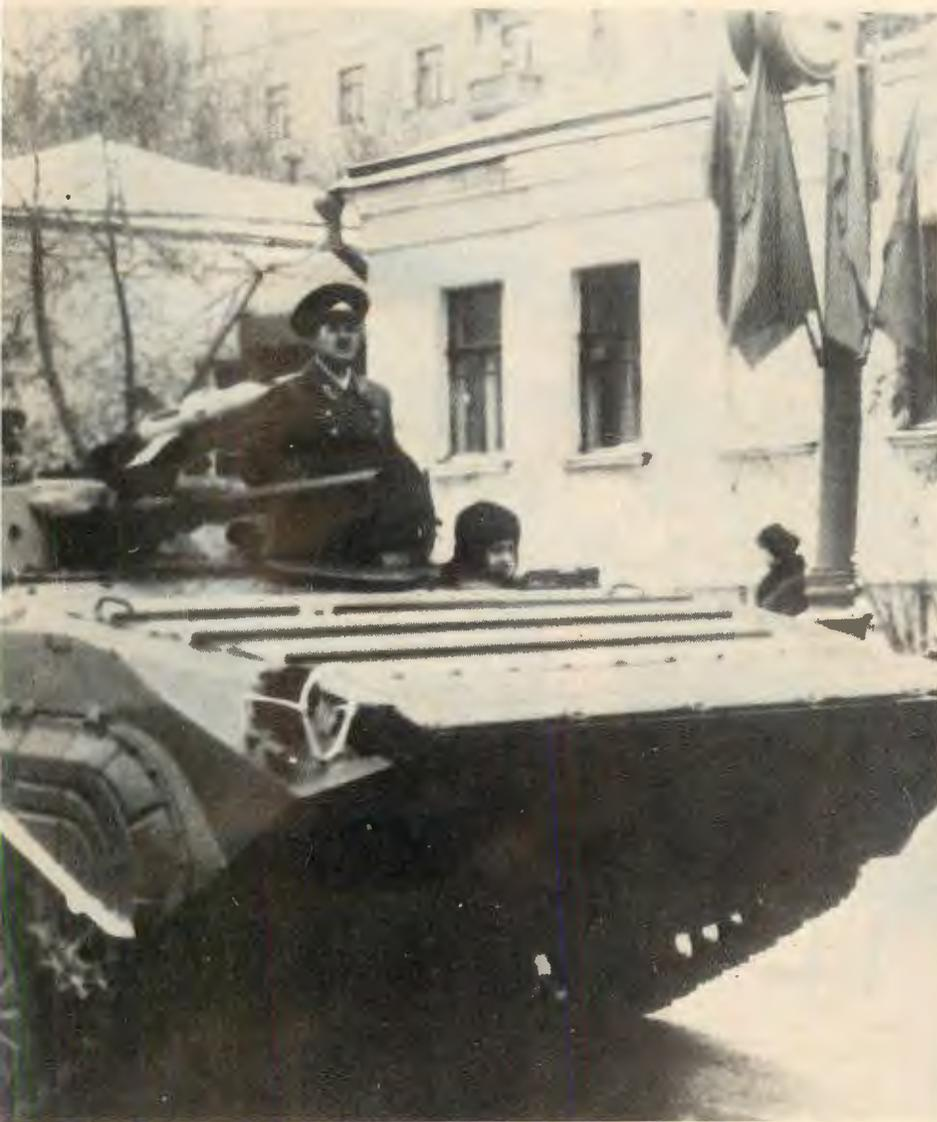
Standard BMP-A IFV, armed with 73mm cannon, shows powerful combination of cannon, machine gun, anti-tank guided missiles and rifle squad in Moscow parade. Photo: U.S. Army
